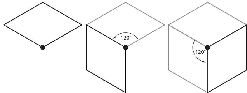
When the basic shape of the object (here: a cube) is drawn, the corresponding faces can simply be created by a double  $120^\circ$  rotation of the shape.
