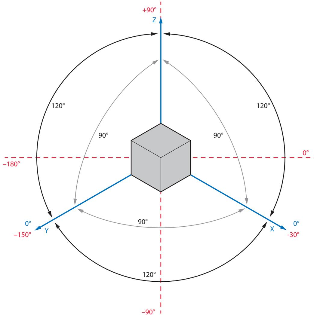
Isometric projections are a two-dimensional drawing of three-dimensional objects, created by a parallel projection. Objects look like having a volume, without actually having one.
