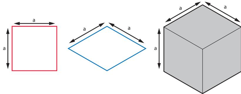
Dimension **a** (x, y) of the quadratic shape (red) can be directly used on the isometric axes x, y (blue).
