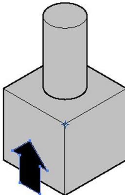
Finally you have created an arrow, which is correctly displayed as an isometric object, positioned in the x/z plane. This arrow fits to any other object, which is drawn as an isometric body.
